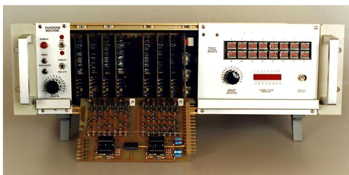
One of the eight printed circuit cards of the Pangram Machine, bearing two counters and the resistor fan-outs for letters R and S. At left, two groups of three LEDs signal current counter positions.
