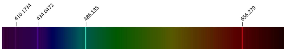
Reference emission spectrum of hydrogen (H), restricted to the wavelengths of visible light.
