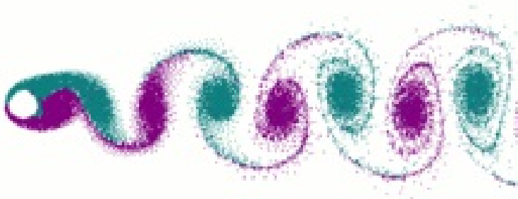
Laminar and turbulent flow in a cigarette's smoke.
